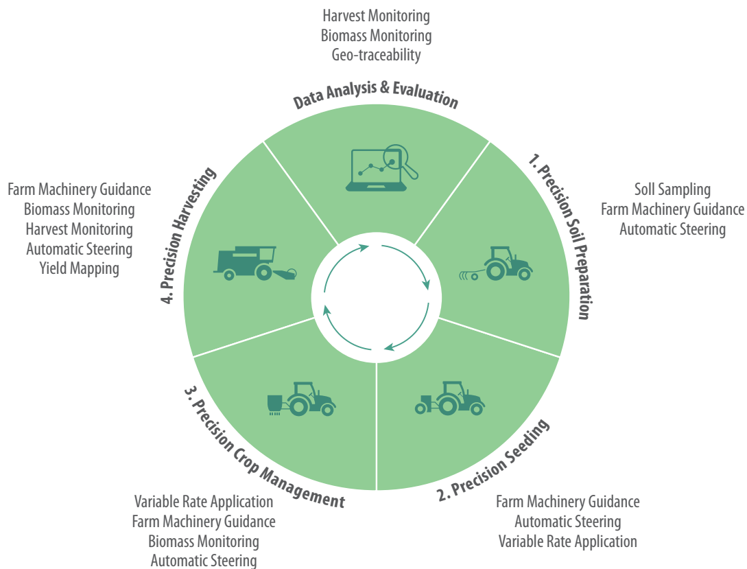
Figure 4: Overview of GNSS-supported precision agriculture activities along the crop cycle (adapted from CEMA 30 )
